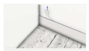
By pulling the textile tab, the tape is stretched and loses its adhesive power. In this way the JUUNOO Glue is pulled from between the skirting board and the wall panel.
