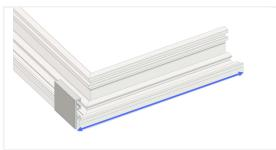
Cut and fix the base profiles at a 45° miter (or other desired angle). Measure the snap-in profile to be cut and use a leftover snap-in profile to identify the exact over measurement.
