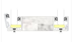
Clear the glass on the inside and vacuum the acoustic felt. Place the second layer of glass like the first layer.
