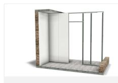
Mark the doorway on the back of the click panels. Do the same for each panel adjacent to the door. Saw off any excess. Make sure to leave a small gap between the panel and door frame (see below)
