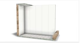
Put the rest of the panels in place. Use an extra strip of JUUNOO tape for the last panel.
