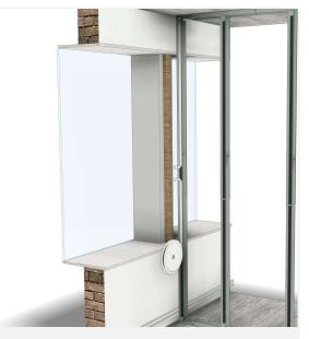
Fix a wooden bar to the window to support the click-in panel. Apply JUUNOO tape to the C-module.
