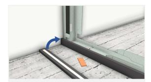
Glue a black MDF strip (30x10 mm) to the bottom of the modules using double-sided adhesive tape. This creates a shadow gap.
