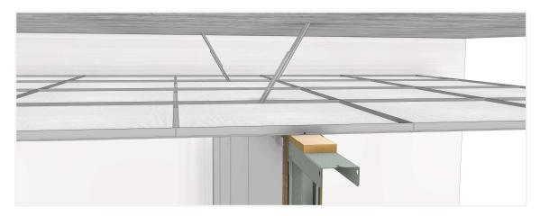
3) Some ceilings have a U-channel where a bolt (M6 or smaller) connects the modules.
