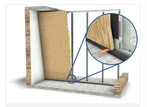
Place the wooden board on the shadow gap and level the board using shims. Then press the panel against the modules.
