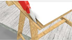
After installing the first click panel, cut off a piece of the groove of the  $2^{nd}$  panel.
