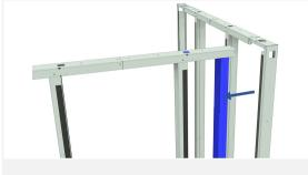
Position the angled structure, but do not fix the adjacent C-module (blue) yet; slide it into the left.
