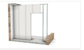
Screw the plasterboards to the structure using self-drilling screws. The drill point ensures that no collar forms around the holes. This increases the reusability of the modules.
