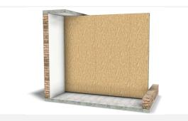
Finish the wall. Break off the shims under the panels, leaving a small piece under the panel. This ensures that the panel does not start to sag.
