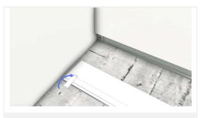
Fold the tab in half over the tape to create a small loop protruding from the skirting board.
