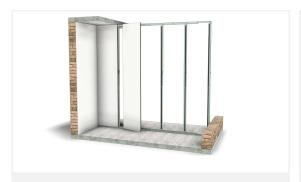
Apply the  $2^{nd}$  panel at an angle of  $\pm 30^{\circ}$ .
