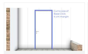
If the door frame has an architrave, the click panels do not have to be perfectly aligned with the frame. A margin of 4 cm is possible. In any case, ensure that the panels do not touch the door frame so that acoustic leak is avoided.
