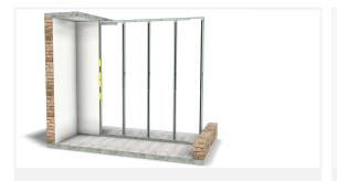
The panels are not placed directly on the floor to avoid possible problems with rising damp.
