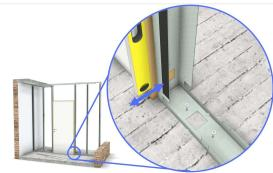
Level the bottom of the C-module on the hinge side and fix the base.
