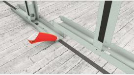
In order to be able to disassemble it easily later, we recommend cutting the tape at the joint of each module.
