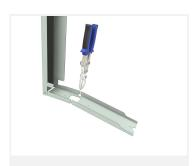
Cut the raised edges on the horizontal profile at the mark indicated.
