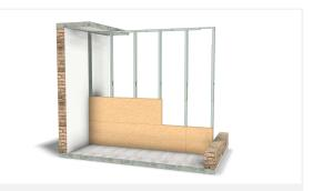
Attach the next panels, using the remainder of the right panel as the start of the first panel. There is no need for the joint to be over a vertical strut.
