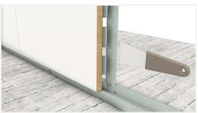
The rest of the click panels can be loosened with a straight spatula. Insert this between the panel and the module.
