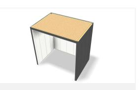
Fill the top edge of the ceiling with OSB.
