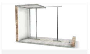
Insert the I-modules. Insert a door top profile in the place of the door opening.
