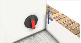
Hook the putty knife behind the click panel and score it up and down while pulling the panel backwards (using a suction cup if necessary).
