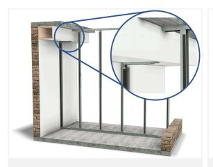
Fix the C-module under the recess. Ensure the I-module is level. You may need to cut a piece of this.
