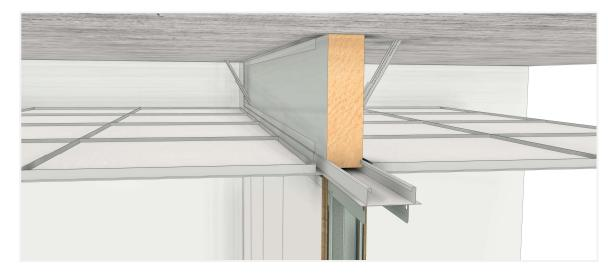
For an alternative arrangement, the drop ceiling can be installed after the installation of the JUUNOO wall. This is a more robust structure, but less easy to adapt.
