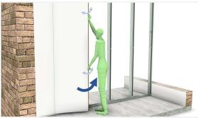
The tongue of the 2<sup>nd</sup> panel hooks into the groove of the first panel. Move back and forth until closed.
