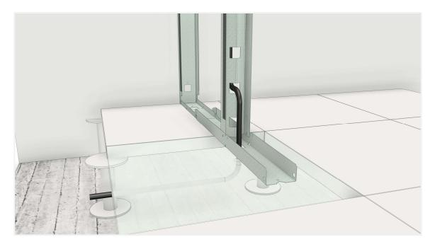
Cables can run above and below the vertical profiles; the maximum height between the horizontal and vertical posts is 39 mm.
