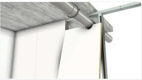
From the 3<sup>rd</sup> panel, make a cut-out for the pipe with a tolerance of 3 mm. Apply it from below, but do not press it against the tape of the I-module yet.
