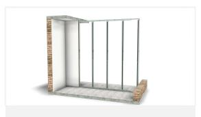
Saw the first panel to the right size and attach it, perfectly vertical, onto the modules.
