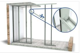
Attach the telescopic cross section to the C-modules at the desired height. The cross profile has a flap that can be fixed with self-tapping screws.
