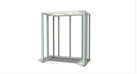
Position and fix all C-modules except the 2 to be placed against the rear wall
