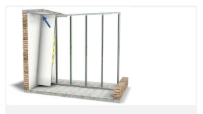
Install the first panel against the left wall and ceiling. Do not press the panel against the tape yet.
