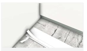
Insert a section of the textile tab under the tape. Make sure that the tab on the other side of the tape sticks out a little.
