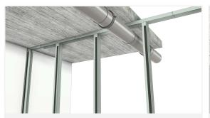
Insert all modules. In most cases, piping comes between the studs and you can attach the horizontal profiles above the pipes to the ceiling.
