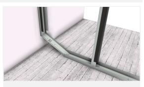
Insert the C-module into the I-module.
