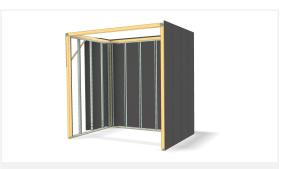
Attach the outer BaseClick panels to the modules. These will ensure the structure is rigid.
