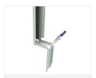
Fold the profile piece over and cut the bottom edge.
