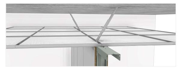
2) If the wall is not to be placed on a profile of the drop ceiling, a wooden board can be first fixed to the ceiling and then all the modules will be positioned against it.
