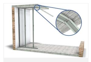
Click the large 120 cm door profile (= 2 I-modules) into the I-modules and fix it.
