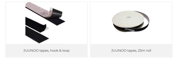
The JUUNOO tapes should be installed on a dust-free, degreased surface, at a temperature above 20 °C and at a humidity between 40% & 60%. After assembly, the JUUNOO tape must be pressed on firmly. The JUUNOO tape should be allowed to rest for at least 24 hours before loading.
