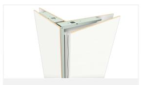
Apply sealant to the 'legs' of the corner profile, where there is contact with the panel. The profile does not need to be glued to the C-module.
