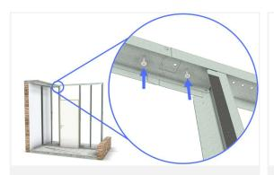
Finally, fix the C-module to the door strike side. Put a wooden block in between if necessary.
