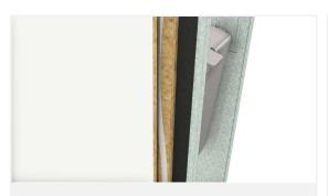
Apply a fine line of transparent silicone glue in the groove.
