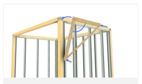
Temporarily brace the structure at right angles.
